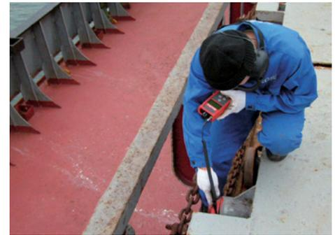
Ultrasound leak detector (ULD)
